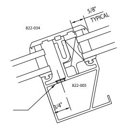
3/8"° ACCESS HOLE W/ GROMMET FOR WIRING IN RAFTER (SEE D06)
