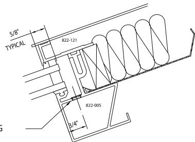
3/8"° ACCESS HOLE W/ GROMMET FOR WIRING IN RAFTER (SEE D06)
