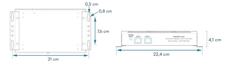
Figure 1: Wall Mounting Hole Pattern
